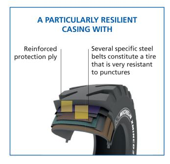
A substantial crown and robust shoulders reinforced with a protection band make a tire that is particularly resistant to impact ruptures, cuts and tread tearing
