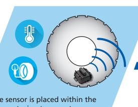
The sensor is placed within the tire, capturing temperatures and pressures in real time.
