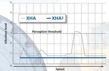
**TEST CONDITIONS:** Loader power: 200 kw Total weight unloaded: 26 000 kg Total weight loaded: 35 500 kg Tyre size: 26.5 R 25 XHA2 Tyre Pressure: Front: 3.75 bar Rear: 2.25 bar
