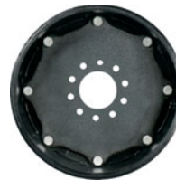
Hub Adapter MSPN 31119 CAI 076712 12 mm thick 1015 carbon steel / reversible 3.68" (93.5 mm) center dia. 10 x 140 mm bolt pattern 0.63" (16 mm) bolt holes, tapered Fits Moffett M5500 Truck Mounted Forklift
