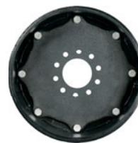
Hub Adapter MSPN 31119 CAI 076712 12 mm thick 1015 carbon steel / reversible 3.68" (93.5 mm) center dia. 10 x 140 mm bolt pattern 0.63" (16 mm) bolt holes, tapered Fits Moffett M5500 Truck Mounted Forklift
