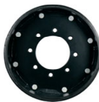
Hub Adapter MSPN 47868 CAI 291074 12 mm thick 1015 carbon steel / reversible 6.0" (152.4 mm) center dia. 8 x 8.0" bolt pattern 0.67" (17 mm) bolt holes, tapered Use adapter to change offset on 8 x 8.0" standard fitment size
