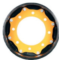
Hub Adapter MSPN 47139 CAI 419992 12 mm thick 1015 carbon steel / reversible 9.0" (228.6 mm) center dia. 8 x 10.91" bolt pattern 0.79" (20 mm) bolt holes, no taper Fits front of Case backhoe loader machines
