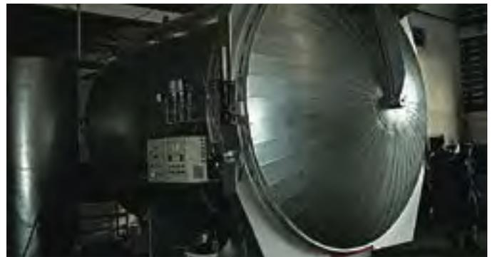
Curing in an autoclave
