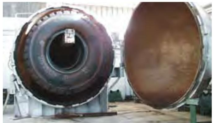
Curing in autoclave
