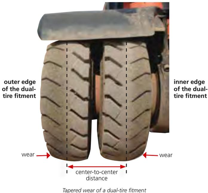
The tires in the same dual-tire fitment sometimes show “tapered” wear: the outer edges of the tires in the dual-tire fitment are worn more than the inner edges.
