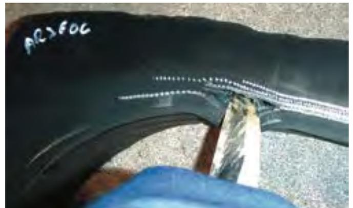
Separation of the components in a tire
