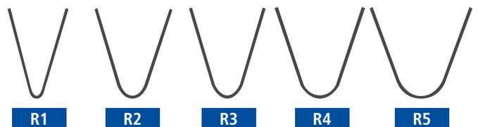
**Only "R3"-type rounded blades are generally used for earthmover tires.**
