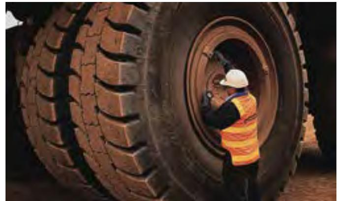
Clean the valve before checking the pressure
