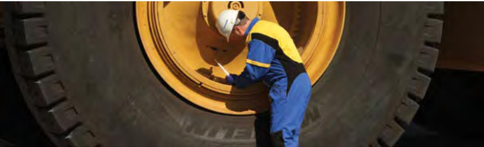
Inspecting the bead of a mining tire
