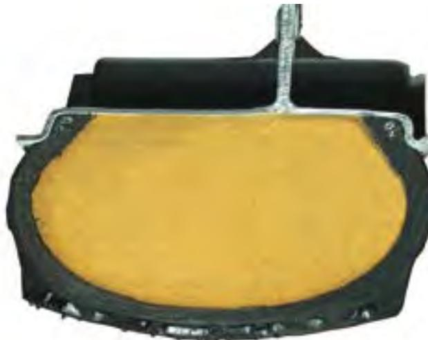
*Polyurethane elastomer solid fill*
