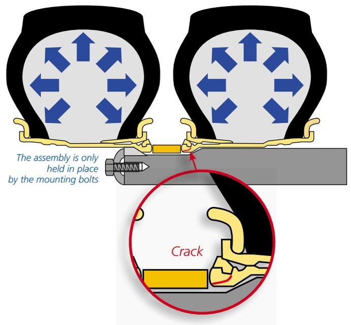
*The assembly is only held in place by the mounting bolts*
