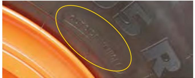
Tire mounted with the "Outside vehicle" marking visible
