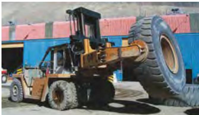
Forklift truck equipped with tire handler
