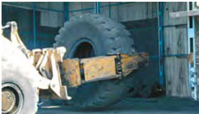
Loader equipped with tire handler
