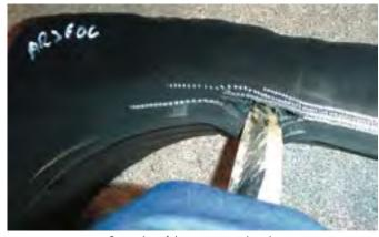
Separation of the components in a tire
