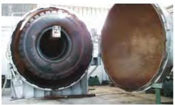
Curing in autoclave
