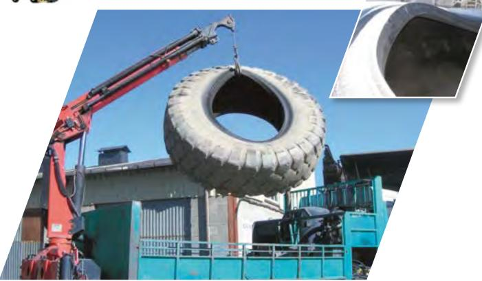
Incorrect handling may cause irreparable damage
