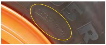
Tire mounted with the "Outside vehicle" marking visible
