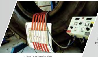
Curing using sectional press
