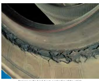
Damage on the bead due to overloading of the vehicle
