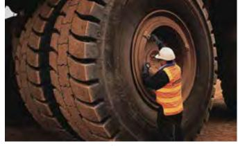
Clean the valve before checking the pressure
