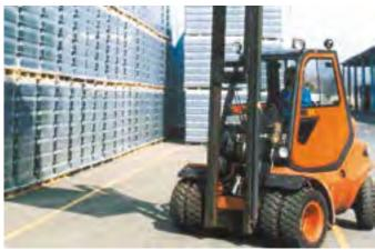
Forklift truck fitted with dual tires
