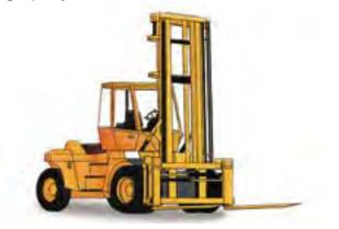
Front axle always the drive axle, rear axle always the steering
