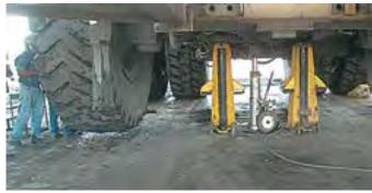
Alignment is adjusted with the wheels off the ground
