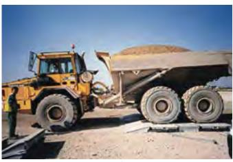
Weighing the rear axles of an articulated dumper
