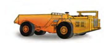
Tilting dump body or fixed dump body fitted with an ejector. Articulated machine.
