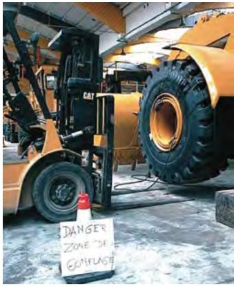
Inflation with tire vertical, with surrounding area protected in case of ejection of rim components
