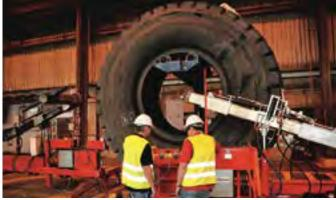
Curing with a thermopress
