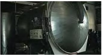
Curing in an autoclave
