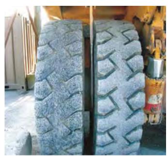
Do not mount tires with different degrees of wear on a dual-tire fitment
