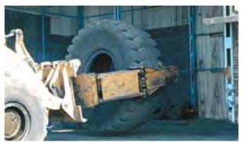
Loader equipped with tire handler
