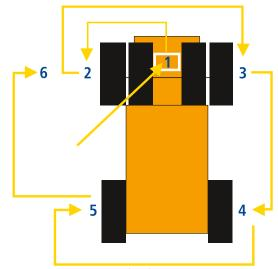
Inspecting the tires on a forklift truck with telescopic mast
