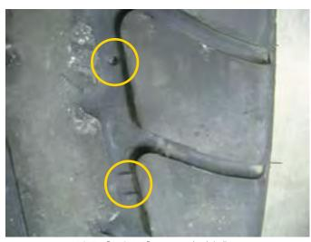
MICHELIN® X-CRANE®: regroove depth indicator (at the top), tire wear indicator (at the bottom)
