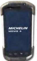
MEMS® (Michelin Earthmover Management System) is the first remote pressure and temperature monitoring system for mining machine tires.
