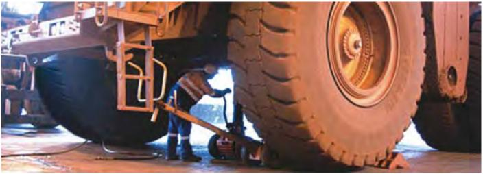
To adjust the suspension, the vehicle must be placed on blocks
