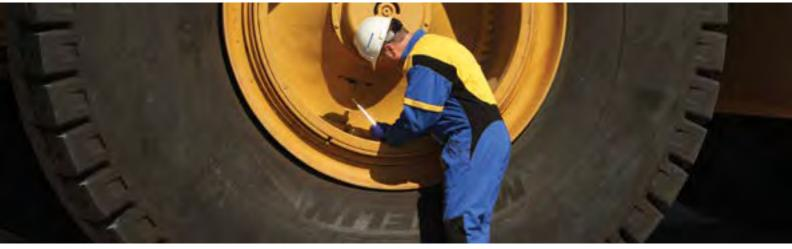
Inspecting the bead of a mining tire
