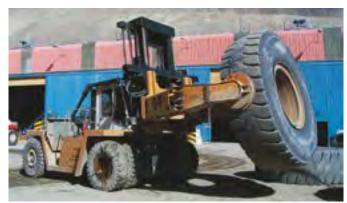
Forklift truck equipped with tire handler
