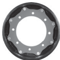
Hub Adapter MSPN 47462 12 mm thick 1015 carbon steel / reversible 9.0" (228.6 mm) center dia. 8 x 10.75" bolt pattern 0.67" (17 mm) bolt holes, tapered Fits some Bobcat machines
