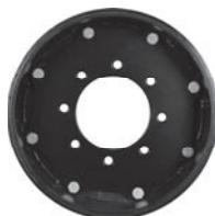
Hub Adapter MSPN 47868 12 mm thick 1015 carbon steel / reversible 6.0" (152.4 mm) center dia. 8 x 8.0" bolt pattern 0.67" (17 mm) bolt holes, tapered Use adapter to change offset on 8 x 8.0" standard fitment size
