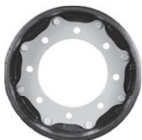
Hub Adapter MSPN 47139 12 mm thick 1015 carbon steel / reversible 8.75" (222.3 mm) center dia. 8 x 10.91" bolt pattern 0.79" (20 mm) bolt holes, no taper Fits front of Case backhoe loader machines
