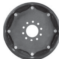
Hub Adapter MSPN 31119 12 mm thick 1015 carbon steel / reversible 3.68" (93.5 mm) center dia. 10 x 140 mm bolt pattern 0.63" (16 mm) bolt holes, tapered Fits Moffett M5500 Truck Mounted Forklift
