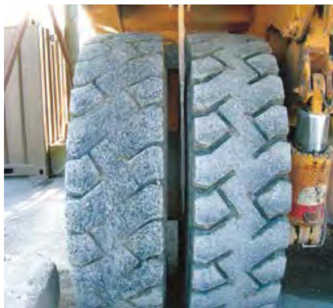
Do not mount tires with different degrees of wear on a dual-tire fitment
