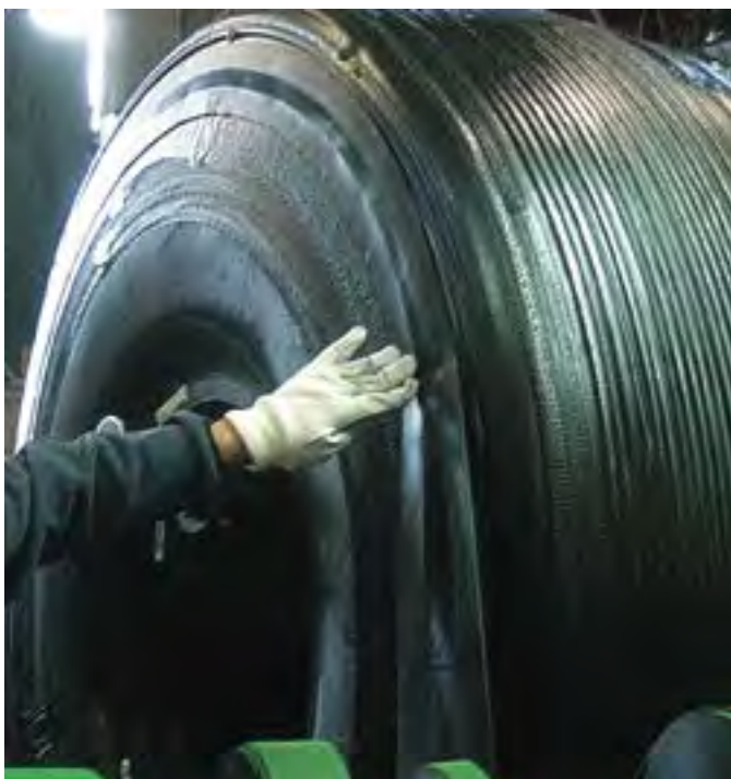
Applying layered strips
