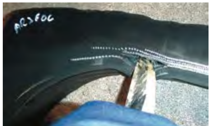
Separation of the components in a tire
