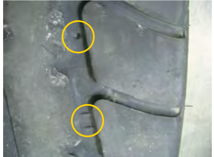
MICHELIN® X-CRANE®: regroove depth indicator (at the top), tire wear indicator (at the bottom)
