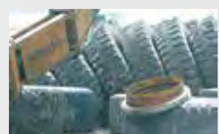
8 Remove the bead seat band and the flange
