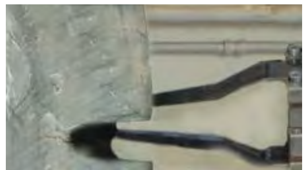
Regrooving extends the life of the tire
