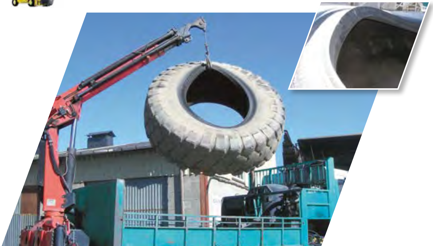
Incorrect handling may cause irreparable damage
