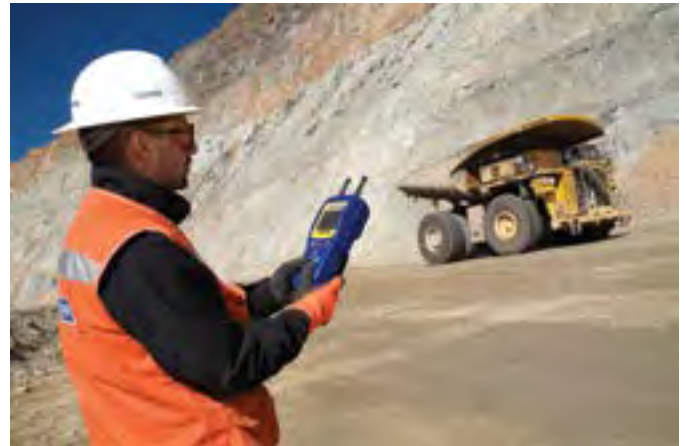
With MEMS, you can check the pressure of the tires remotely without having to stop the machines
