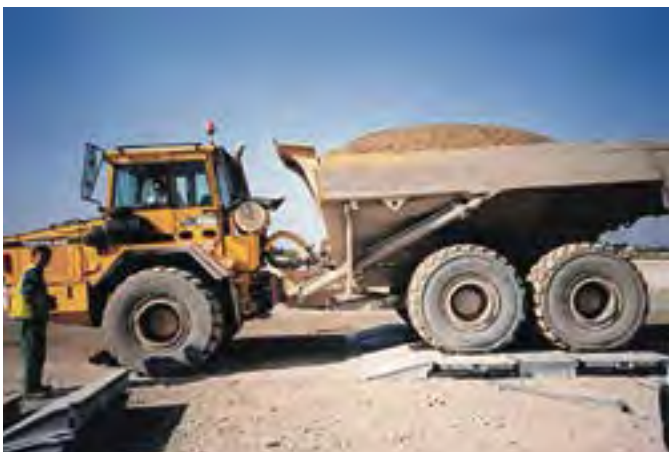
Weighing the rear axles of an articulated dumper
