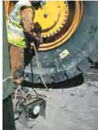
Tighten the nuts in accordance with the manufacturer's instructions
