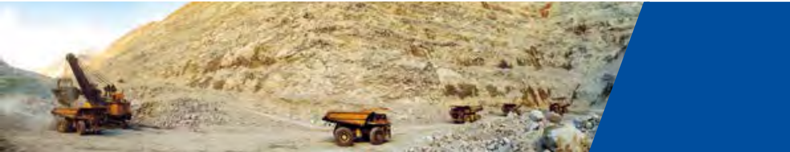
Regular maintenance of loading areas helps to extend the service life of tires
