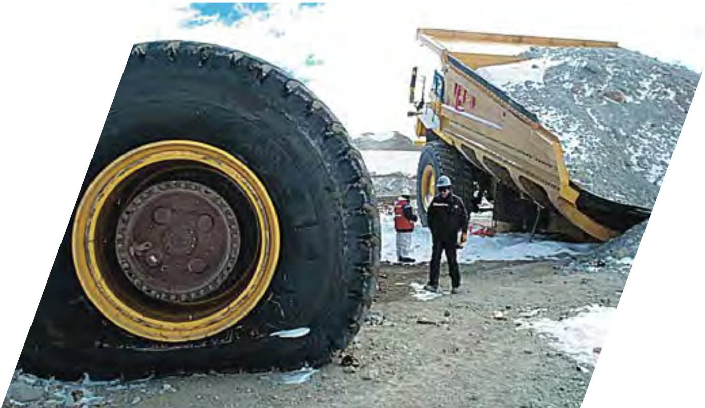
The projection of all the tire/rims component has effects that are a great deal more dangerous and destructive than just a burst tire
