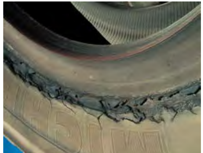
Damage on the bead due to overloading of the vehicle
