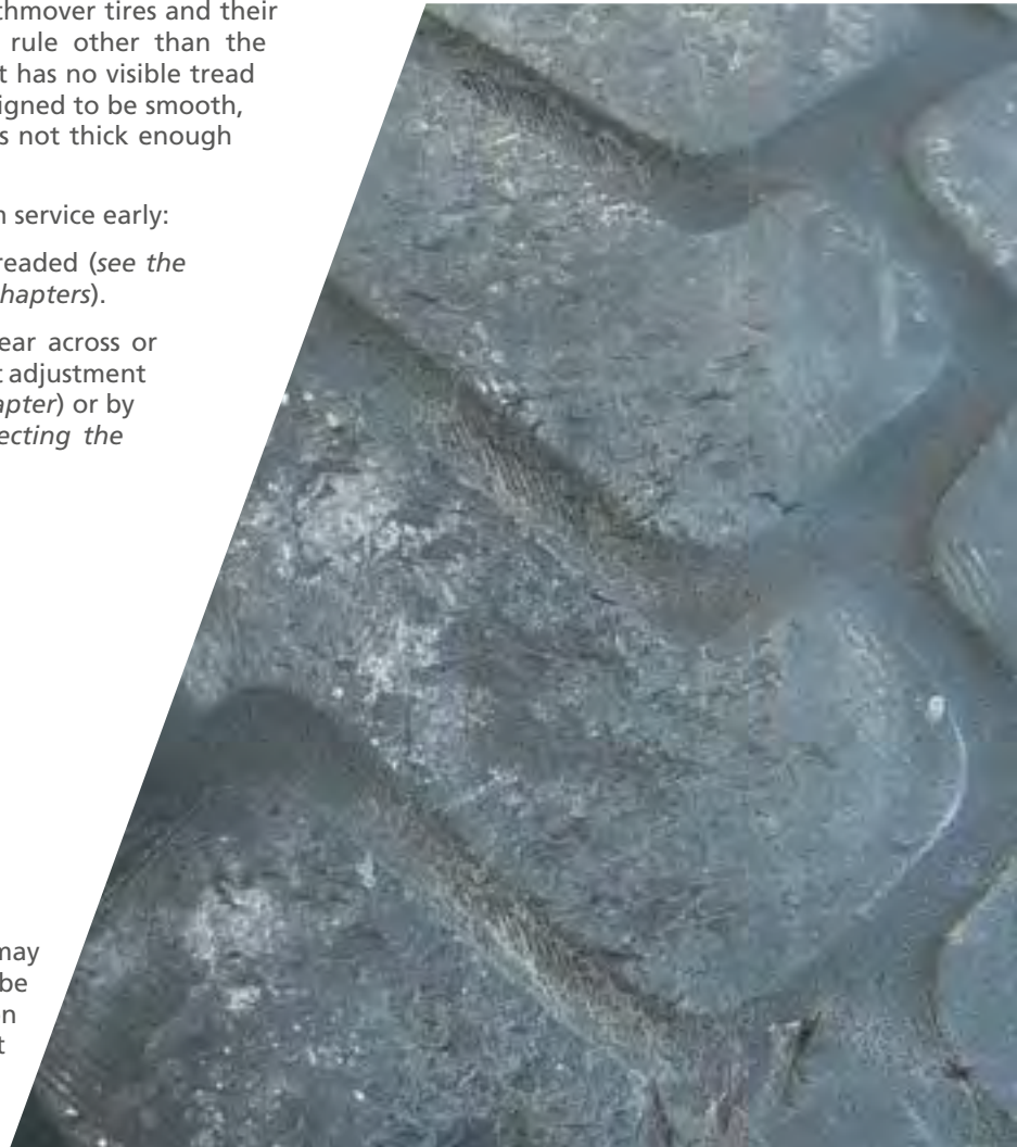
Remove the tire when there is no tread pattern left
