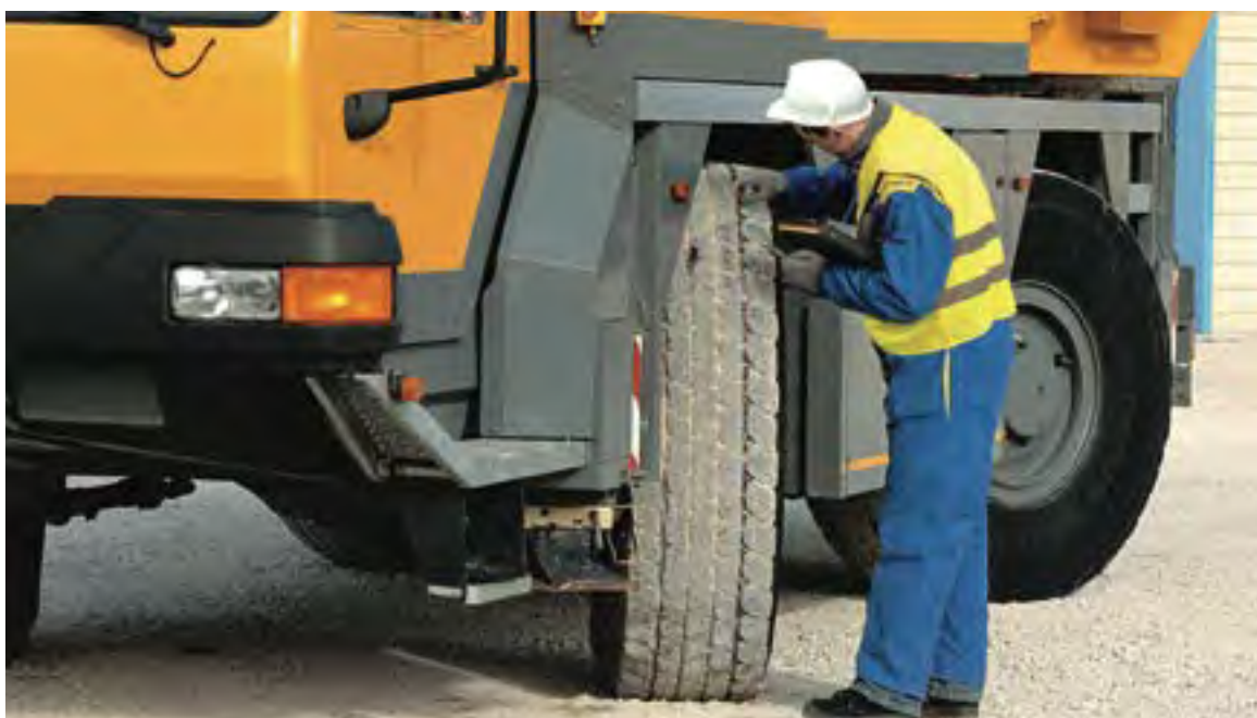
Start with the left front tire, then work around the vehicle
