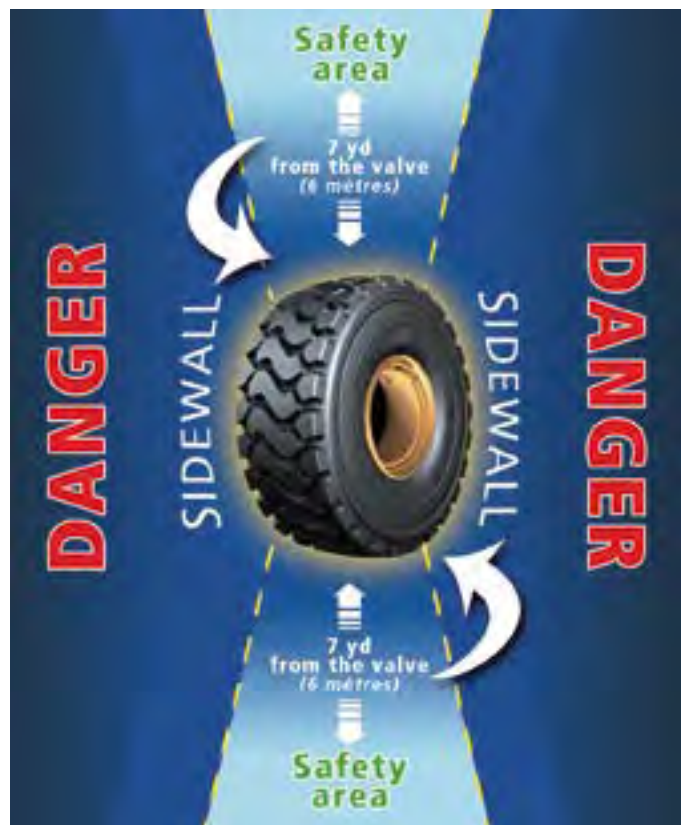
Always stand facing the tread during inflation
