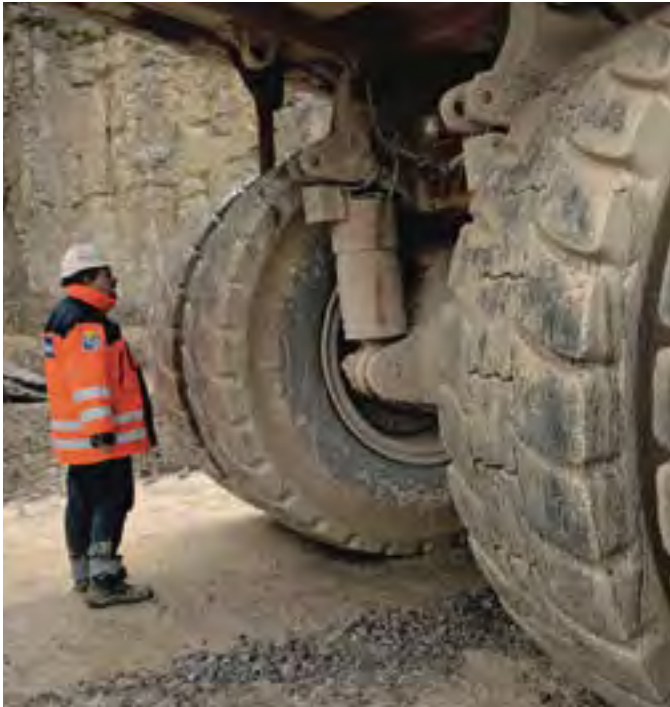
Regular inspection of dual-tire fitments is essential
