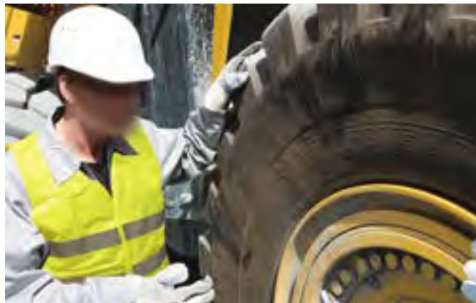
Check the appearance of the tread
