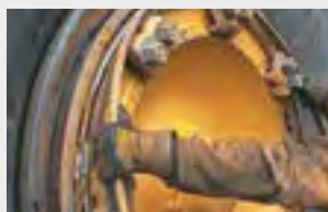
11 Fit the locking ring
