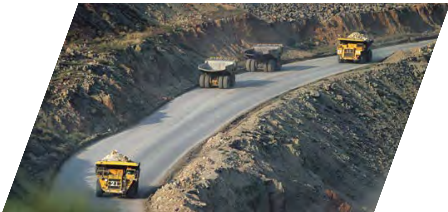
Long cycles increase the risks of overheating (with comparable loads and at comparable speeds)
