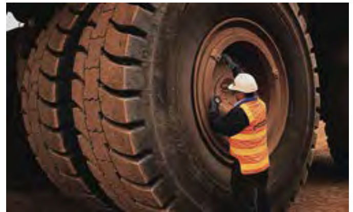
Clean the valve before checking the pressure
