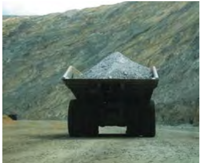
A load that is off-center can cause a specific overload on one side
