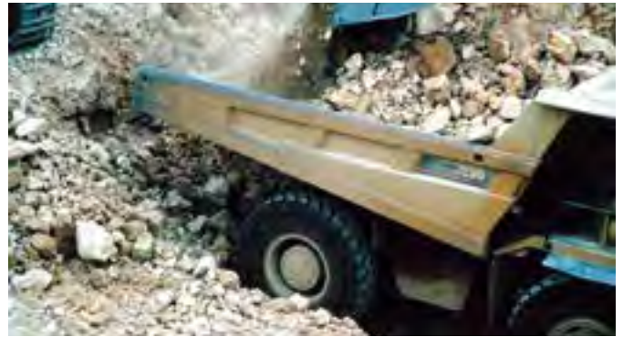
There is an increased possibility of tread blocks being torn off on stony surfaces
