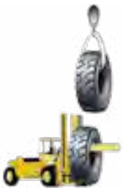
Holding the tire too tightly may distort it
