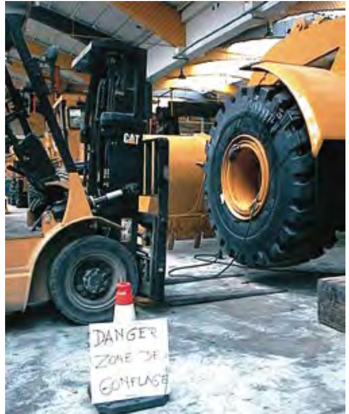
Inflation with tire vertical, with surrounding area protected in case of ejection of rim components
