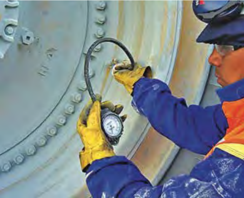
Keep to the recommended inflation pressure
