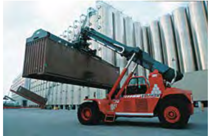
On reach stackers, the steering wheels (rear) are subjected to greater stresses even when loaded
