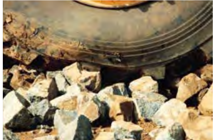
Traveling over stones significantly reduces the service life of tires
