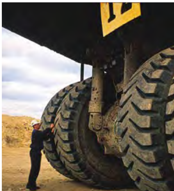
Check there are no objects trapped between the tires of a dual tire unit
