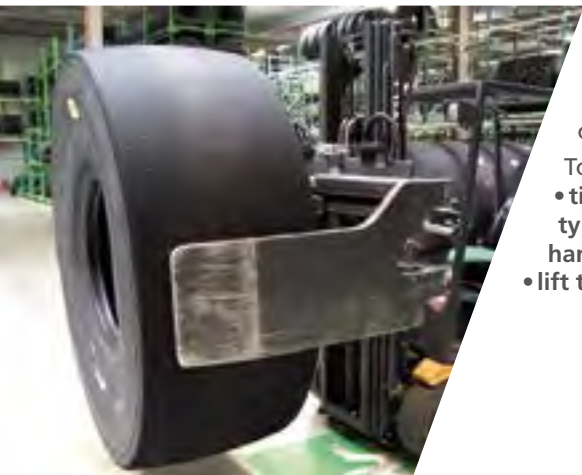
Holding the tire too tightly may distort it
