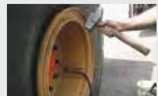
12 Inflate and lightly tap the locking ring
