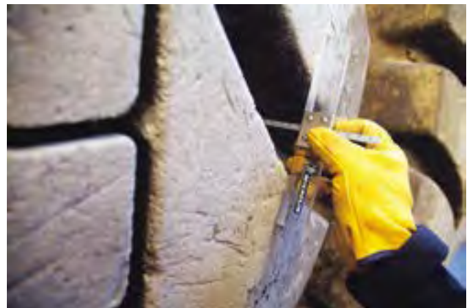
Measure the remaining tread depth at the indicated locations, in several places
