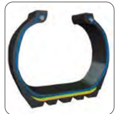
Radial construction separates the work of the crown from that of the sidewalls
