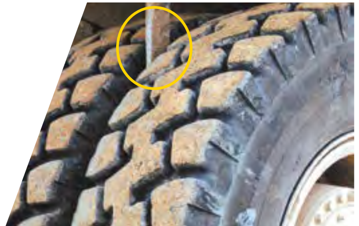
Dual-tire fitments must be protected by a rock ejector
