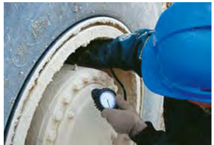
The pressure when cold must not differ from the recommended level by more than +/- 10%
