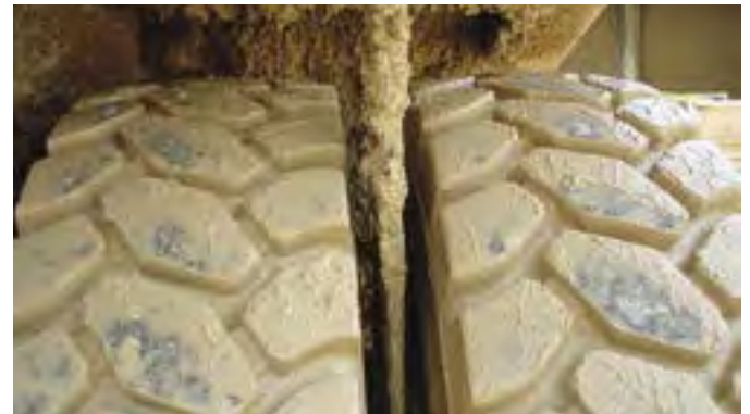
Check the rock ejectors
