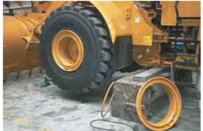
Using blocks to immobilize a loader
