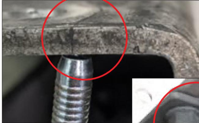
Figure 3. Examples of head unit cracking along flange
