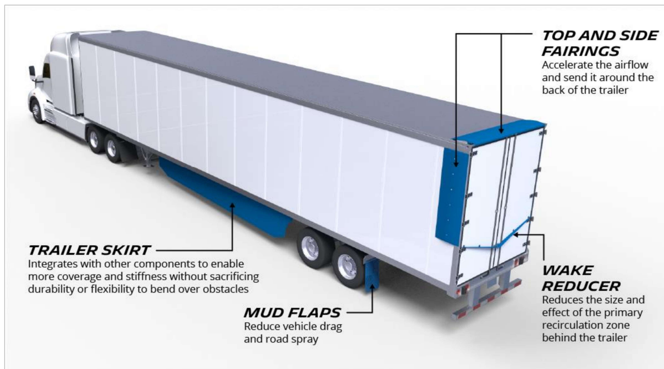
Figure 1: MICHELIN® Energy Guard Solution Components
