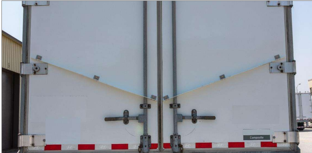
Figure 8: Wake Reducer Installations on Swing Doors
