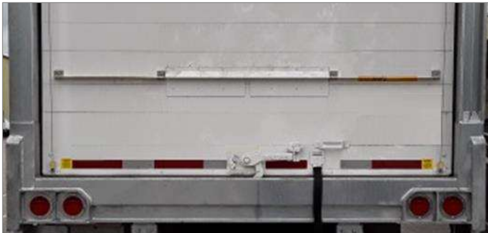
Figure 9: Wake Reducer Installation on a Roll-up Door
