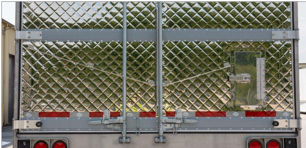
Figure 9: Wake Reducer Installation on a Roll-up Door
