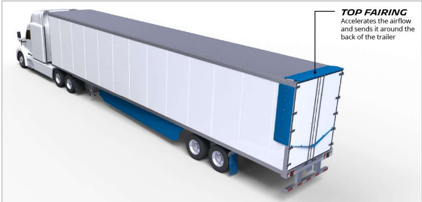
Figure 3: MICHELIN® Energy Guard Solution Top Fairing
