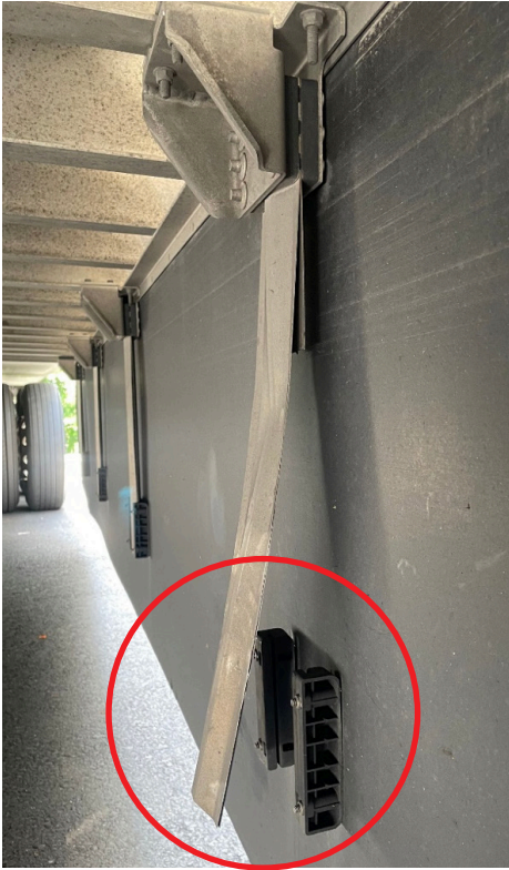
Leaf springs disengaged with damage
