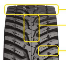
A wide footprint combined with a shallow tread provide low rolling resistance and thus reduced fuel consumption.
