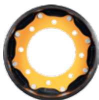
Hub Adapter MSPN 47139 12 mm thick 1015 carbon steel / reversible 8.75" (222.3 mm) center diameter 8 x 10.91" bolt pattern 0.79" (20 mm) bolt holes, no taper Fits front of Case backhoe loader machines
