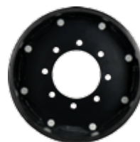
Hub Adapter MSPN 47868 12 mm thick 1015 carbon steel / reversible 6.0" (152.4 mm) center diameter 8 x 8.0" bolt pattern 0.67" (17 mm) bolt holes, tapered Use adapter to change offset on 8 x 8.0" standard fitment size
