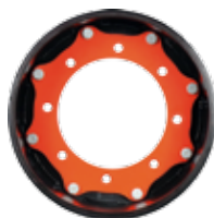
Hub Adapter MSPN 47462 12 mm thick 1015 carbon steel / reversible 9.0" (228.6 mm) center diameter 8 x 10.75" bolt pattern 0.67" (17 mm) bolt holes, tapered Fits some Bobcat machines
