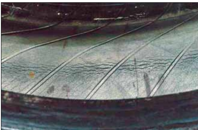
Potential Zipper Rupture
