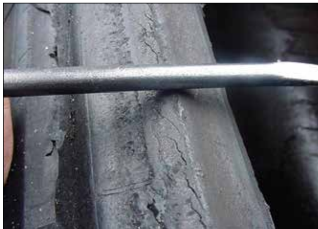
1st Stage – Turning of the Bead
