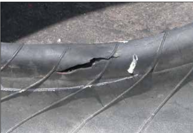
Bead Damage Caused by Mounting/Dismounting
