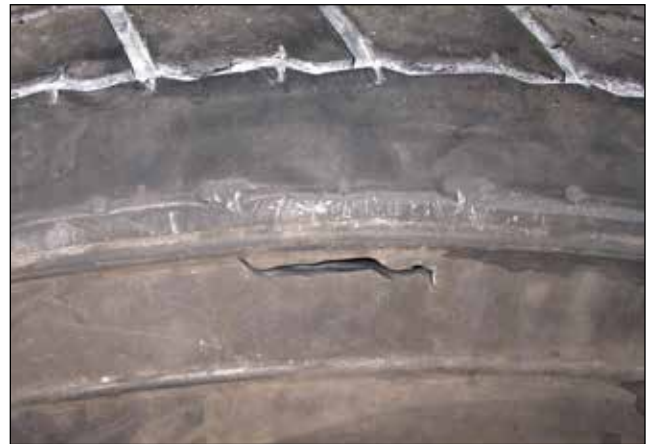
Sidewall Rupture Shock
