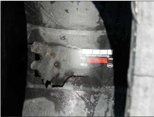
EFFECT: Improper Repair or Improper Repair Procedures CAUSE: Premature Failure of Repair
