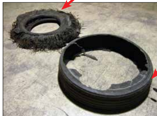
EFFECT: Run Flat CAUSE: Crown Perforation/Penetration
