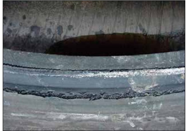
2nd Stage – Bead Splitting from Heat
