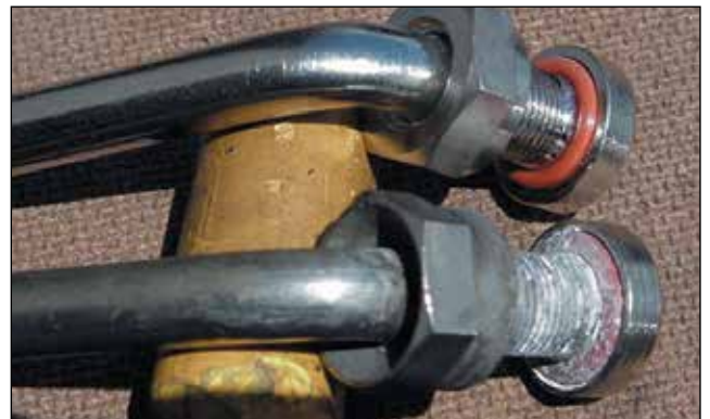
Note Corrosion On Bottom Valve
