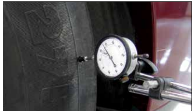
Measuring Lateral Runout on Outside Shoulder
