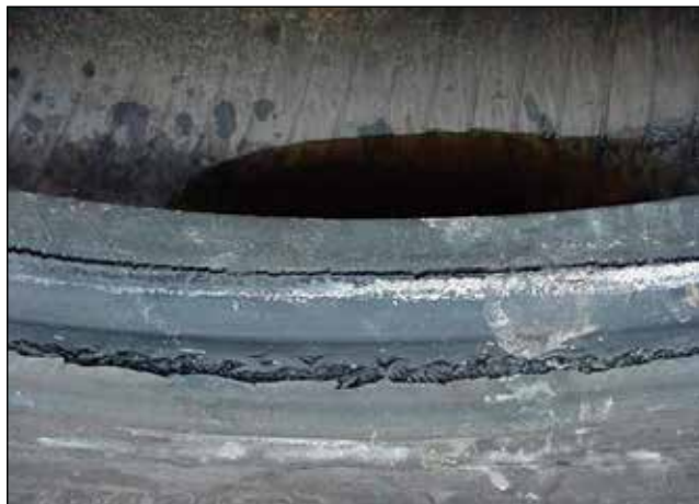
2nd Stage – Bead Splitting from Heat
