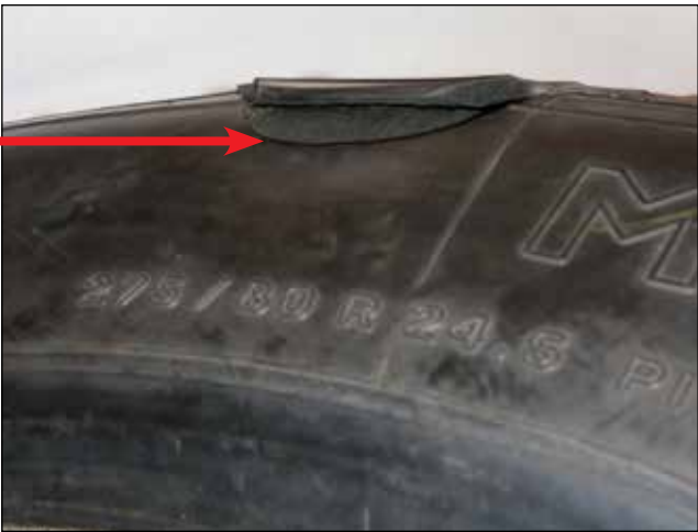
EFFECT: Sidewall Separation Due to Air Infiltration CAUSE: Improper Repair
