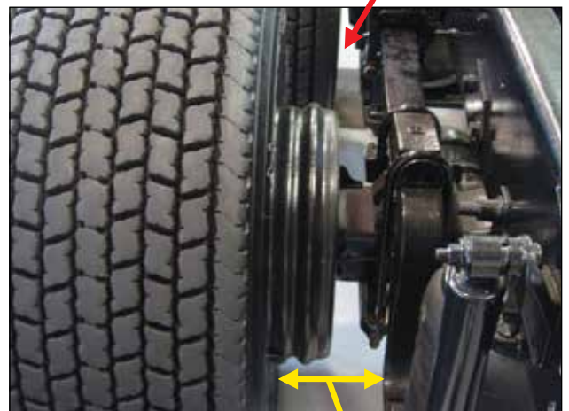
Correct Lateral Clearance
