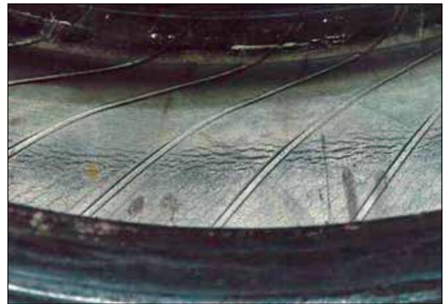
Sign of Run Flat Damage – Interior
