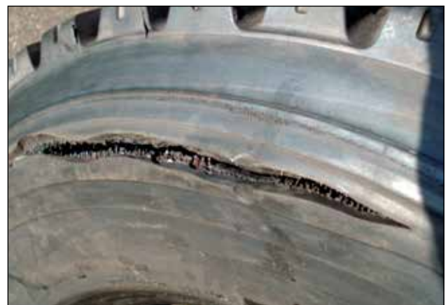
Zipper Resulting from Run Flat Condition
