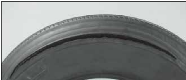
EFFECT: Zipper Rupture CAUSE: Damage/Weakening of Radial Steel Cables as a Result of Underinflation and Running the Tire Flat
