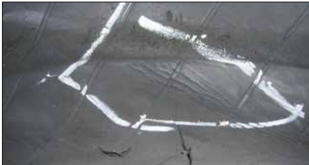
Inner Liner Marbling/Creasing
