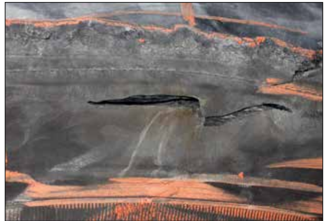
Sidewall Damage from Impact
