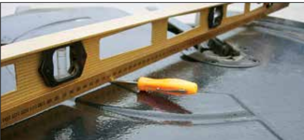
Distortion of the 5th Wheel
