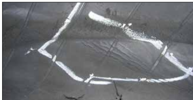
EFFECT: Zipper Rupture CAUSE: Damage/Weakening of Radial Steel Cables as a Result of Underinflation and Running the Tire Flat
