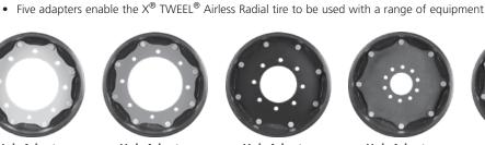
**Hub Adapter Hub Adapter** MSPN 47139 MSPN 47462 CAI 419992 CAI 481115 12 mm thick 1015 12 mm thick 1015 carbon steel / reversible carbon steel / reversible 9.0" (228.6 mm) center dia. 8.75" (222.3 mm) center dia. 8 x 10.91" bolt pattern 8 x 10.75" bolt pattern 0.79" (20 mm) bolt holes, no taper 0.67" (17 mm) bolt holes, tapered Fits front of Case backhoe Fits some Bobcat machines loader machines
