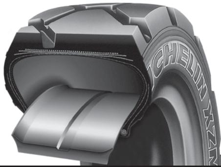
INSTALLATION - CROSS SECTION OF AN INSTALLED TBS
