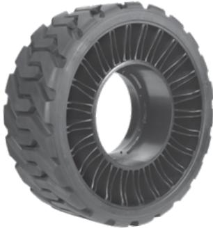
2-Piece Hub X TWEEL SSL shown without a hub adapter installed
