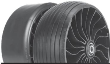
Airless Radial tire designed for the front of mowers.
