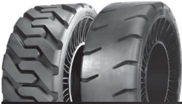
Airless Radial tire designed for skid-steer loaders.
