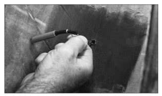
Remove spiral cement tool from the injury and feed the small end of the wire puller through the injury from inside of the tire.
