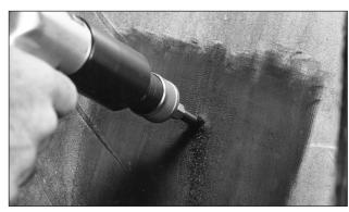
Prepare the injury with the proper size carbide cutter on a low rpm drill (max. 1200 rpm).
