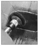
Use a low rpm (max. 5000 rpm) buffer and texturizing wheel to mechanically buff the stem flush to the inner liner. Then buff the outlined area to achieve an even RMA-1 or RMA-2 buffed texture. Use a clean, soft wire brush, remove all dust and debris from the buffed area.
