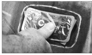
With the tire beads in a relaxed position, center the repair unit over the filled injury. Press the repair unit down into place over the injury. Make sure the directional bead arrows on the repair unit are aligned with the beads of the tire, and press into place. Roll the protective poly back to the outer edges of the repair unit. This enables you to handle the repair unit without contaminating the bonding gum layer. You are now ready to stitch the repair.
