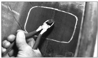
Remove the template and cut off the stem 1/8 inch (3 mm) above the inner liner on the inside of the tire. NOTE: If you do not have a repair template, go to this step and cut the stem; then using the correct sized patch and centering it correctly on the injury – arrows towards the beads – draw your perimeter approximately 1/2 inch larger than the repair patch.
