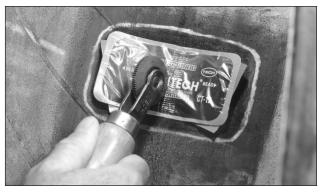
Stitch the repair unit, firmly pressing down from the center toward the outer edges. This will eliminate trapping air under the repair unit.
