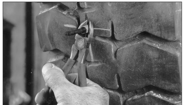
**18** Cut the stem off on the outside of the tire 1/8 inch (3 mm) above the tire's surface. The tire is now ready to be returned to service.
