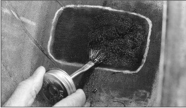
**13** Using Chemical Vulcanizing Fluid (cement), brush a thin, even coat into the clean textured area. Allow 3 to 5 minutes to dry; the vulcanizing cement should be tacky. Areas with high humidity may require a longer dry time. Make sure the cement used is compatible with the repair units you are installing.
