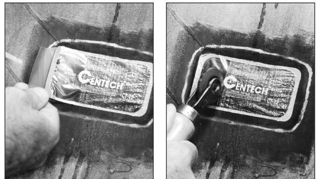
**16** Remove the rest of the poly backing. Stitch the repair unit from the center to the outer edges. Remove the top clear protective poly.
