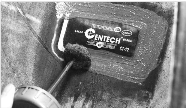
**17** To cover over-buffed areas in tubeless tires, apply Security Sealer to the outer edge of the repair unit and over-buffed area. If tube-type, cover the repair with Tire Talc to prevent the repair from vulcanizing to the tube.
