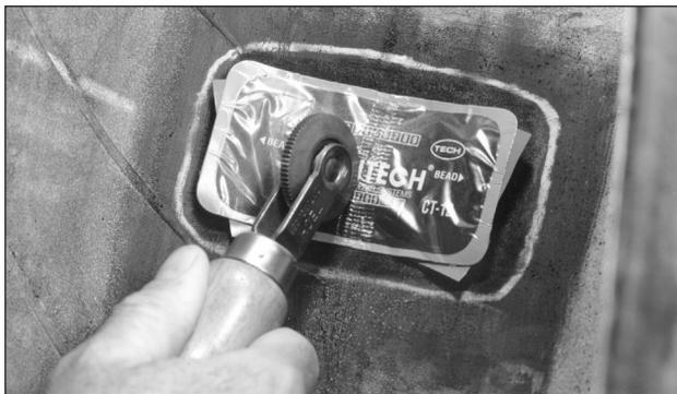
**15** Stitch the repair unit, firmly pressing down from the center toward the outer edges. This will eliminate trapping air under the repair unit.
