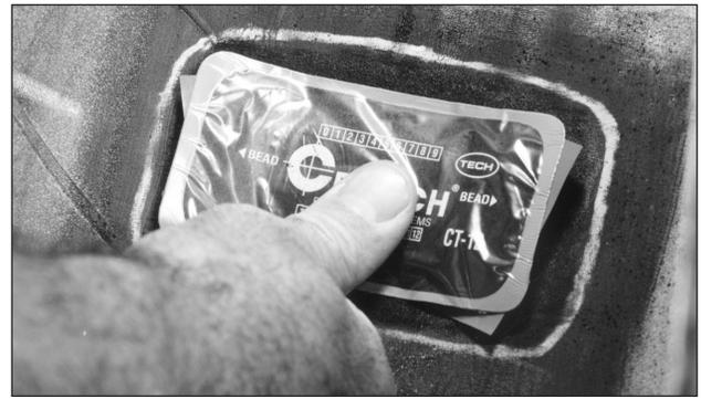
**14** With the tire beads in a relaxed position, center the repair unit over the filled injury. Press the repair unit down into place over the injury. Make sure the directional bead arrows on the repair unit are aligned with the beads of the tire, and press into place. Roll the protective poly back to the outer edges of the repair unit. This enables you to handle the repair unit without contaminating the bonding gum layer. You are now ready to stitch the repair.
