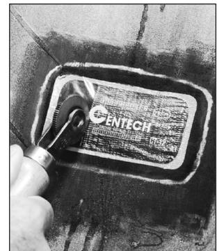
**16** Remove the rest of the poly backing. Stitch the repair unit from the center to the outer edges. Remove the top clear protective poly.
