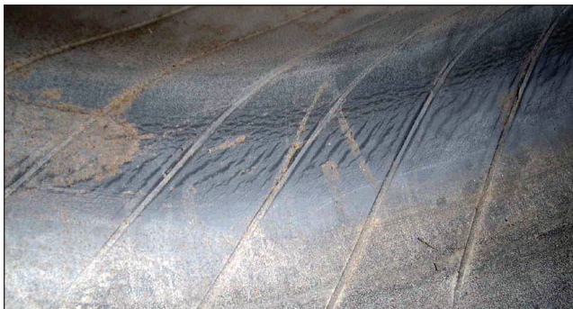
EFFECT: Inner Liner Marbling - Creasing CAUSE: Underinflation
