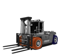
Load wheels Steer wheels Counter balanced forklift truck
