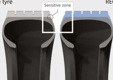
The joint between the belt and the tyre casing outside the sensitive zone.
