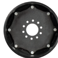
Hub Adapter MSPN 04630 CAI 336820 12 mm thick 1015 carbon steel / reversible 3.68" (93.5 mm) center dia. 10 x 140 mm bolt pattern 0.63" (16 mm) bolt holes, tapered Fits some truck mounted forklifts
