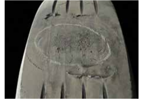
Brake Skid Damage
