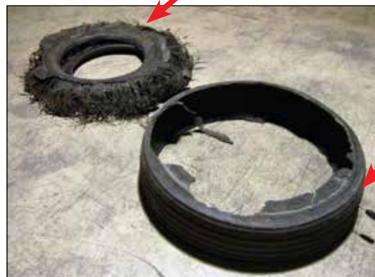
EFFECT: Run Flat CAUSE: Crown Perforation/Penetration
