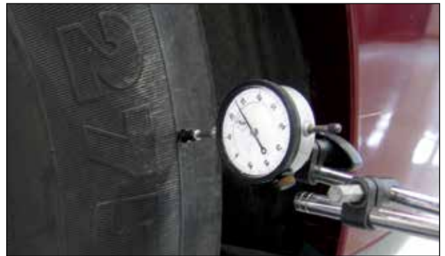
Measuring Lateral Runout on Outside Shoulder
