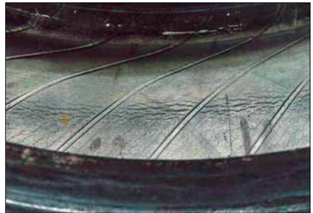
Sign of Run Flat Damage – Interior
