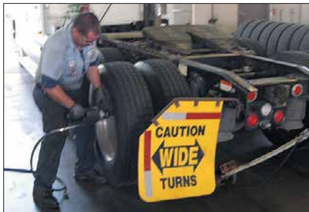
Mounting Dual on the Vehicle
