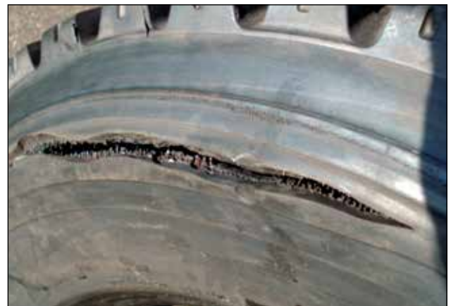
Zipper Resulting from Run Flat Condition
