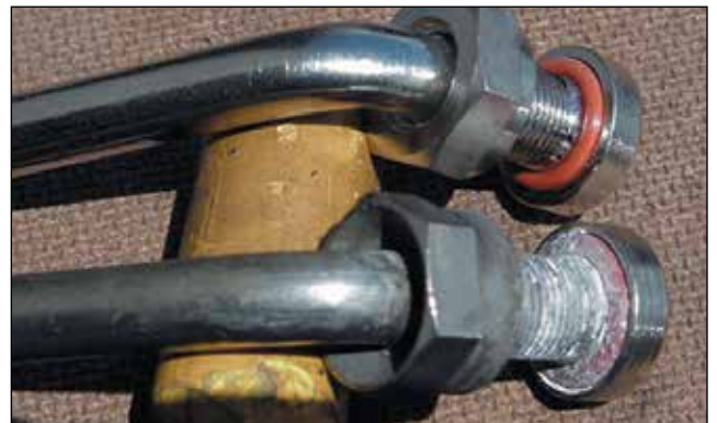
Note Corrosion On Bottom Valve
