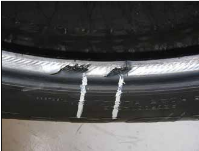
EFFECT: Heating and Deformation of the Bead Rubber CAUSE: Excessive Heat
