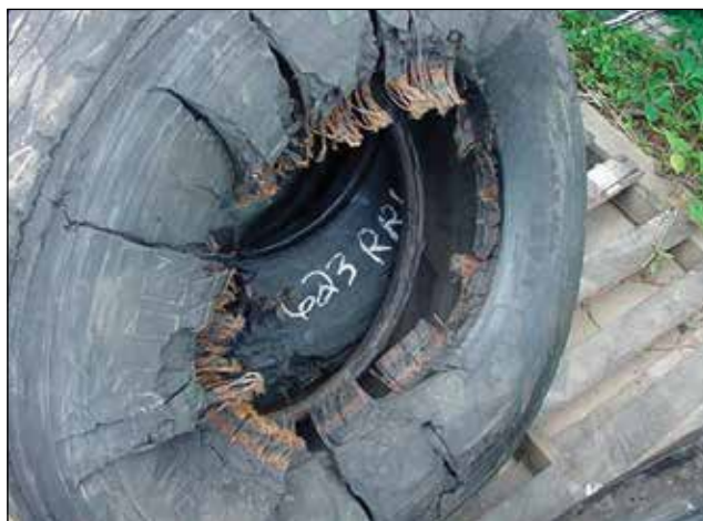
3rd Stage – Complete Unwrapping of the Casing Ply
