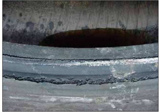
2nd Stage – Bead Splitting from Heat
