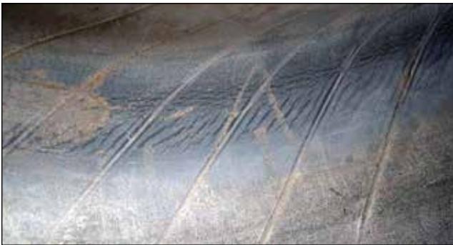
EFFECT: Inner Liner Marbling – Creasing CAUSE: Underinflation
