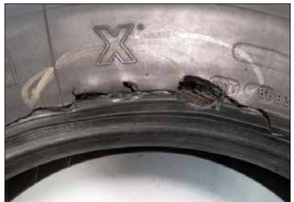
Resulting in sidewall separation and tire destruction from air infiltration.
