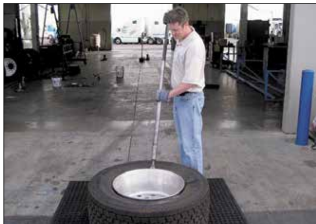
Impact Bead Breaker (Slide Hammer)
