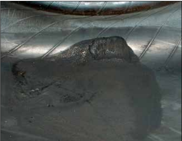
EFFECT: Inner Liner Burn CAUSE: Electrical Discharge Damage
