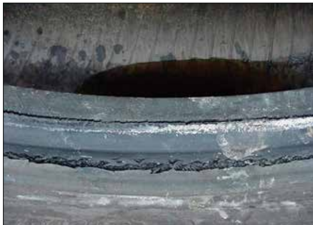
2nd Stage – Bead Splitting from Heat
