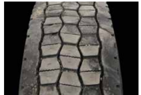
Cupping / Scallop / Alternate Lug Wear
