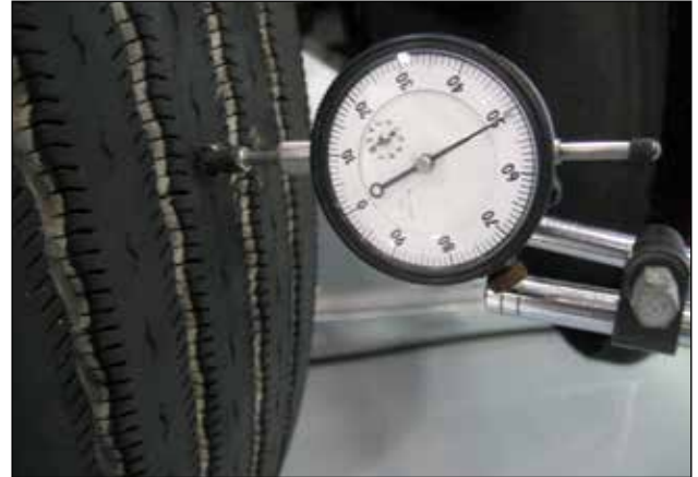
Measuring Radial Runout on Center Rib
