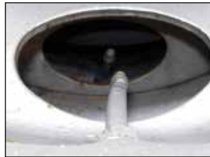
Incorrect Dual Wheel Placement
