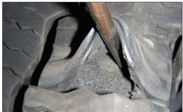
EFFECT: Internal Deterioration of the Tread Rubber CAUSE: Prolonged Use of Dynamometer
