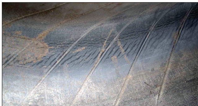
EFFECT: Inner Liner Marbling - Creasing CAUSE: Underinflation
