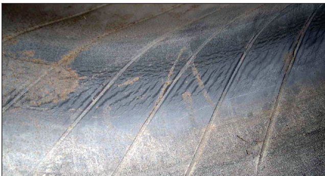
EFFECT: Inner Liner Marbling - Creasing CAUSE: Underinflation
