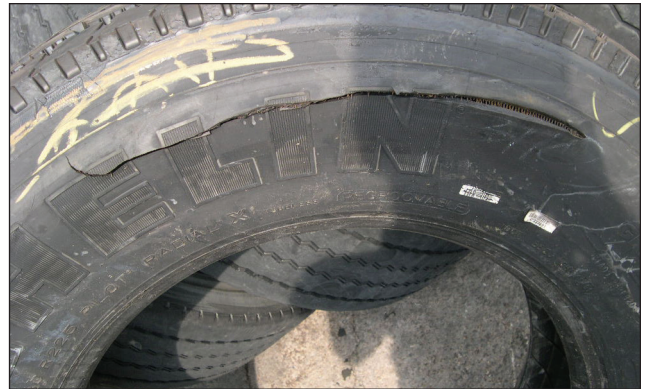
Fatigue Rupture or “Zipper”
