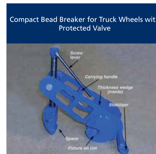
Screw lever / Carrying handle / Thickness wedge - inside / Stabiliser / Spade / Fixture on rim
