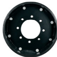
Hub Adapter MSPN 47868 CAI 291074 12 mm thick 1015 carbon steel / reversible 6.0" (152.4 mm) center dia. 8 x 8.0" bolt pattern 0.67" (17 mm) bolt holes, tapered Use adapter to change offset on 8 x 8.0" standard fitment size
