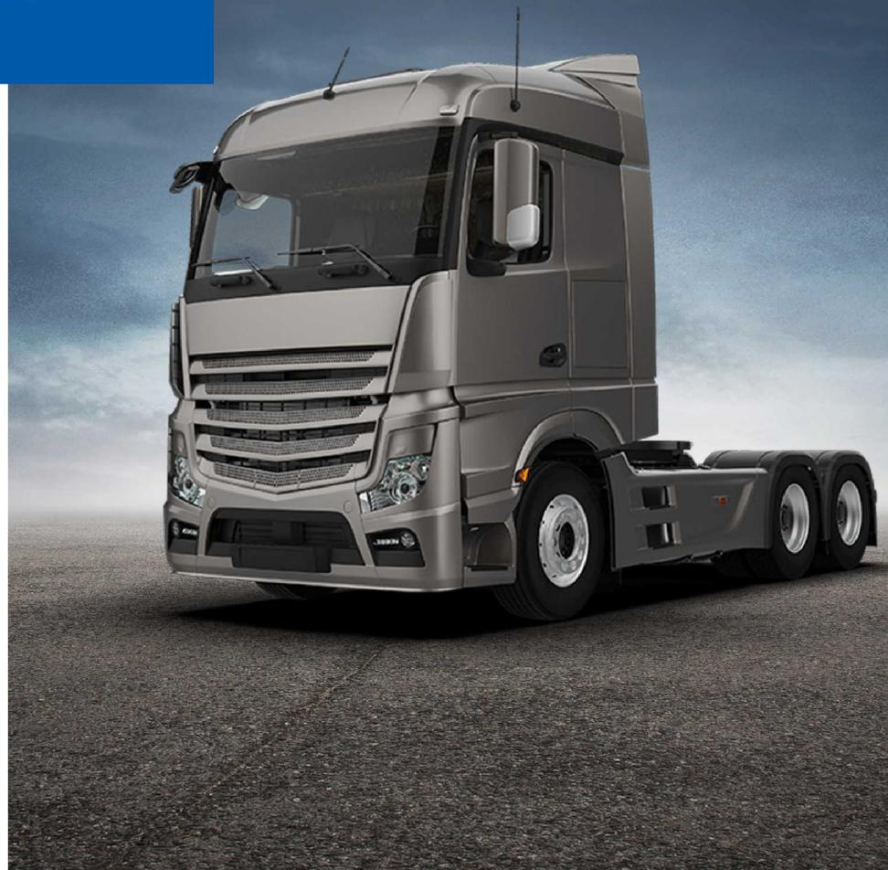
**Wheel Nuts** - Tighten inner and outer wheel nuts to the proper torque. (610 -678 Newton Meters). After **81 to 161 Kilometers** of operation, the torque should be rechecked.
