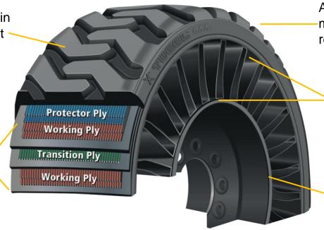
A deep layer of undertread means the core can be retreaded again & again
