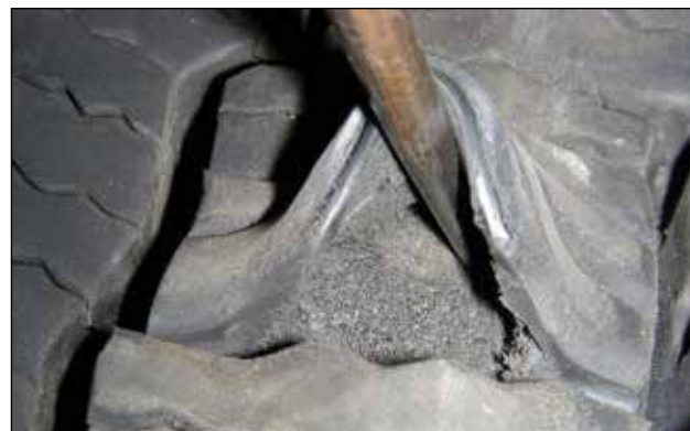
EFFECT: Internal Deterioration of the Tread Rubber CAUSE: Prolonged Use of Dynamometer
