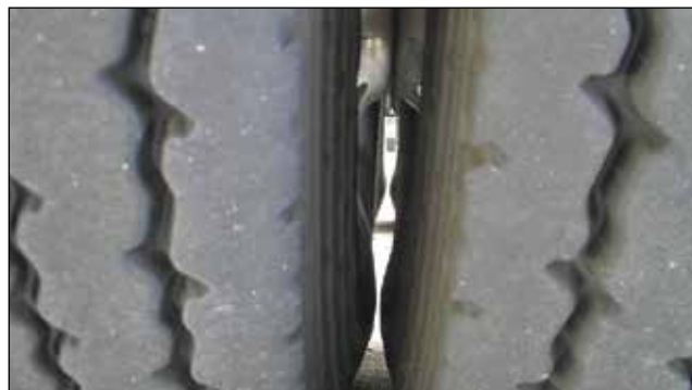
EFFECT: Friction Severely Weakens the Casing CAUSE: Dual Kissing
