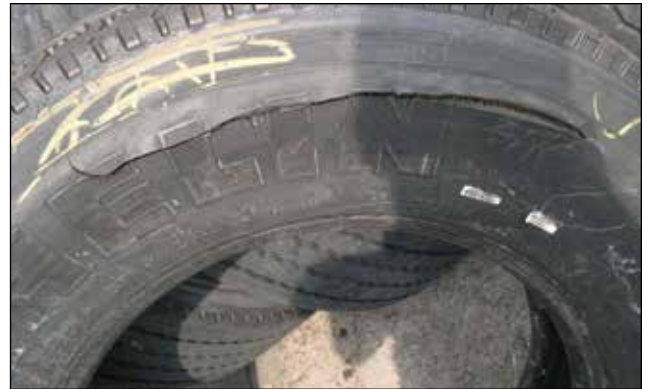
Fatigue Rupture or “Zipper”
