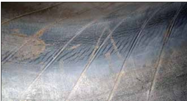
EFFECT: Inner Liner Marbling - Creasing CAUSE: Underinflation
