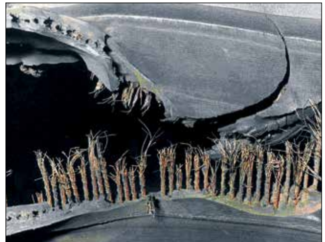
EFFECT: Any Damage That Will Allow the Casing to Oxidize CAUSE: Moisture
