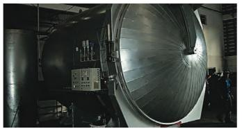
Curing in an autoclave
