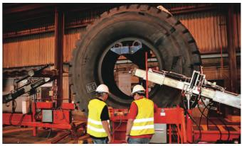
Curing with a thermopress
