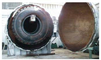
Curing in autoclave
