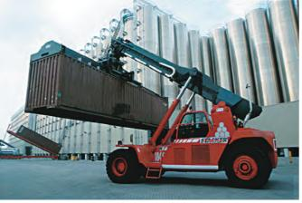
On reach stackers, the steering wheels (rear) are subjected to greater stresses even when loaded
