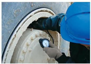
The pressure when cold must not differ from the recommended level by more than +/- 10%
