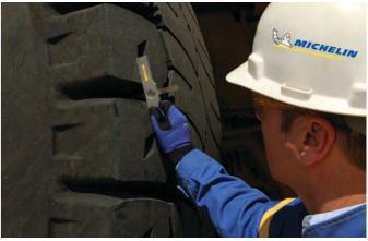
Personal protection equipment must be worr when inspecting the tires on vehicles
