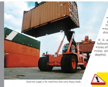
To limit uneven tire wear, vehicles are often fitted with differentials enabling the left dual-tire fitment to rotate at a different speed from that of the right dual-tire fitment.
