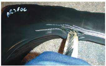
Separation of the components in a tire
