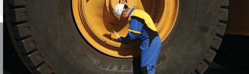
Inspecting the bead of a mining tire
