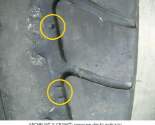
MICHELIN<sup>®</sup> X-CRANE<sup>®</sup>: regroove depth indicator (at the top), tire wear indicator (at the bottom)
