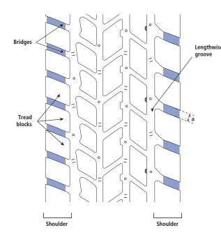
• Remove the bridges on the shoulders (shown in blue) down to the groove base.
