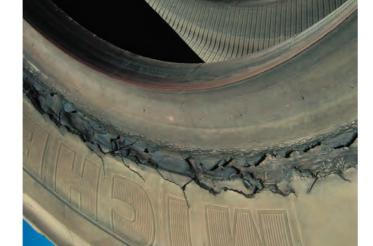
Damage on the bead due to overloading of the vehicle
