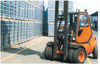
Forklift truck fitted with dual tires
