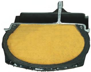
Polyurethane elastomer solid fill
