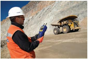
With MEMS, you can check the pressure of the tires remotely without having to stop the machines
