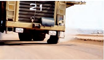
Inappropriate driving damages the tires
