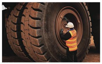
Clean the valve before checking the pressure
