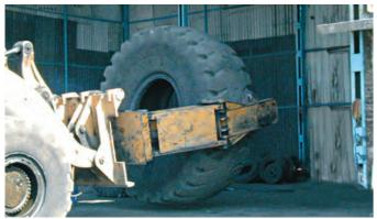
Loader equipped with tire handler
