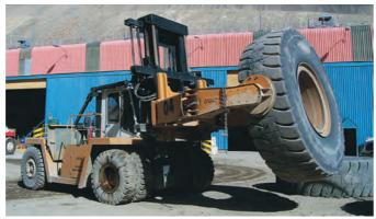
Forklift truck equipped with tire handler
