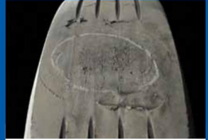
Brake Skid Damage
