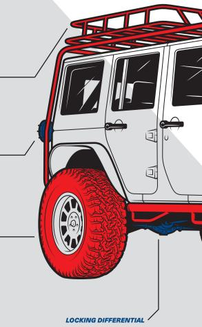
When engaged, a locker distributes equal power to each wheel regardless of the traction the wheel has.
