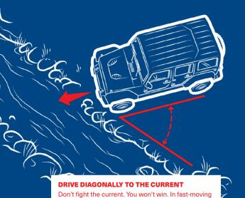
water, it's best to cross at a diagonal to the current. This lessens the amount of surface area for water to
