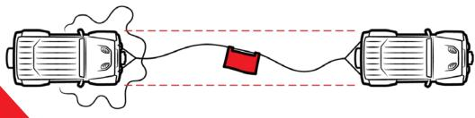
If recovery fails, repeat the process, but give the recovery rope slightly more slack to create more of a whip. The mobile vehicle can also slightly increase its speed.
