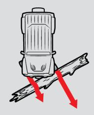
Cross the log at an angle, one tire at a time. This will decrease the clearance needed to cross.
