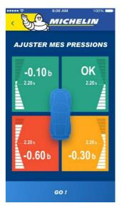
REMINDER: When driving on tracks, it is recommended to always begin a run at the pressures recommended by the manufacturer and to stop after a few laps to adjust the pressure based on the application's recommendations for warm tires. Starting an on-track run when cold with pressures that are too low can harm the integrity of the tire or the vehicle.
