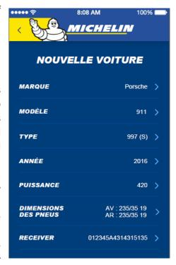
If you want to configure the receiver yourself, make sure that Bluetooth is activated on your phone, that the box is on (connected with the indicator light flashing) and that the telephone and receiver box are close to each other (less than 2 meters). Then press Select on the RECEIVER line, and press ADD A RECEIVER at the bottom of the screen.
