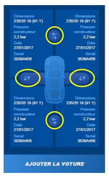
NOTE: Switching from front to rear is only possible for vehicles with exactly the same size tires on the front and rear.
