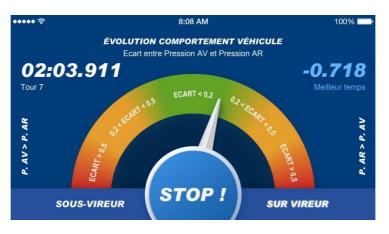
A handling gauge indicates how changes in tire pressure influence changes in your vehicle's balance.
