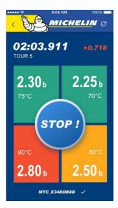
A stopwatch in the top left corner of your screen is automatically set off based on the GPS coordinates of the start line declared in the App. Note that this virtual line may not always correspond to the actual start line of the track itself. This changes nothing regarding the quality of the measurement.
