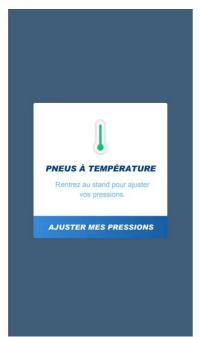
Once all 4 tires are have reached their optimal temperature range, the app indicates that you should go to the pits to correct the pressures in order to get the most out of your tires.
