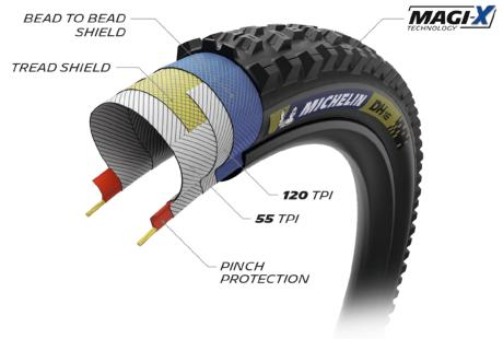
(1) low temperatures: down to 37.4°F (3°C) (2) see cross section of the tire above
