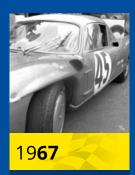
Michelin invents the slick tire at Le Mans, with its smooth tread for better grip on dry surfaces.
