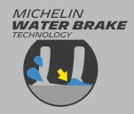
The tread is specifically developed to break up the water film and prevent aquaplaning. The evacuation grooves are reinforced with deep transverse sipes to break up the film of water.
