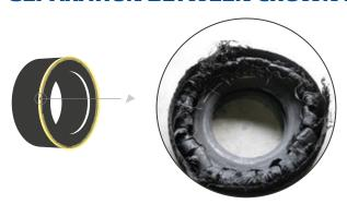
Separation generally begins at the ends of the top layers and may develop into a pocket, or become generalised. Rubber between layers can be reduced to a powder. Sometimes you can observe a sticky rubber appearance. Sometimes shiny cables are evident due to friction. This damage can lead to a sudden loss of pressure or rupture of the carcass ply. This phenomenon can have several causes:
