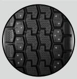
\*Protrusion: length of stud protruding from the tire. The longer the stud protrudes, the better it bites the ice. However, this also increases the risk of tearing or breaking the stud.
