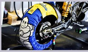
Every machine is delivered with 2 sets of tyre warmers for use with slick tyres, and 1 set of tyres warmers for use with rain tyres.
