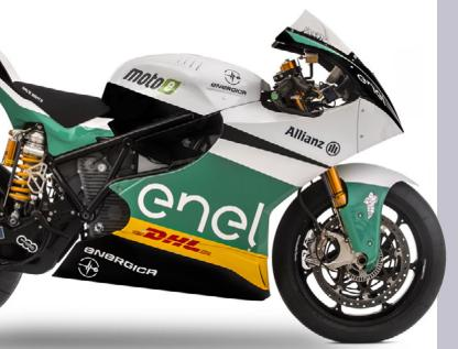
Bike: Energica Ego Corsa Battery capacity: around 20 Kwh **Power:** up to 120Kw (around 160 Hp) Max speed: up to 270km/h Minimum weight: 260kg
