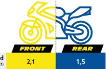
Minimum cold pressure on circuit (1)
